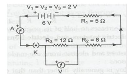
Here ammeter A has been joined in series of circuit and voltmeter V is joined in parallel to 12 ohms resistor.
